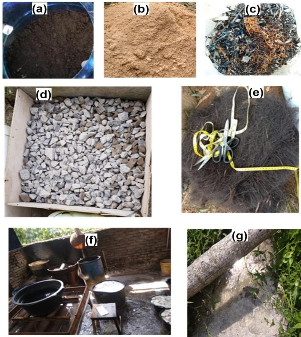
Fig 2. Materials for STBM system, Wastewater Source from Pabrik Tahu and horizon tanah segitiga type STBM system: (A) Local soil, (B) sawdust, (C) iron pellets, (D) split stone, (E) palm fiber, (F) Pabrik Tahu (G) Wastewater from Pabrik Tahu,
